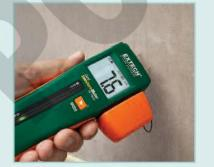
Measures % of Moisture in sheet rock and other building materials using direct pin method. Protective cap snaps onto the side of the housing during use.
